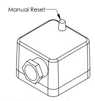
Figure 24: High/Low Gas Pressure Switch
