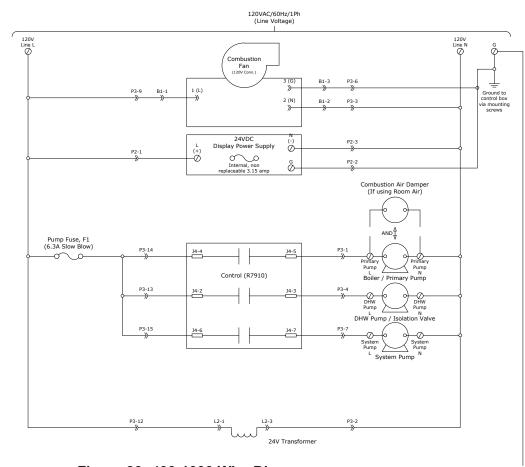
Figure 30: 400-1000 Wire Diagram
