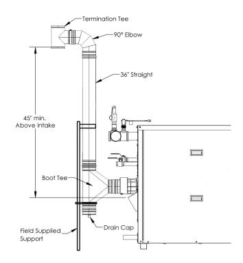
Figure 10: Outdoor Venting Installation
