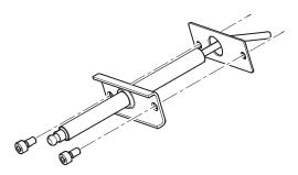
Figure 35: Flame Rod Assembly
