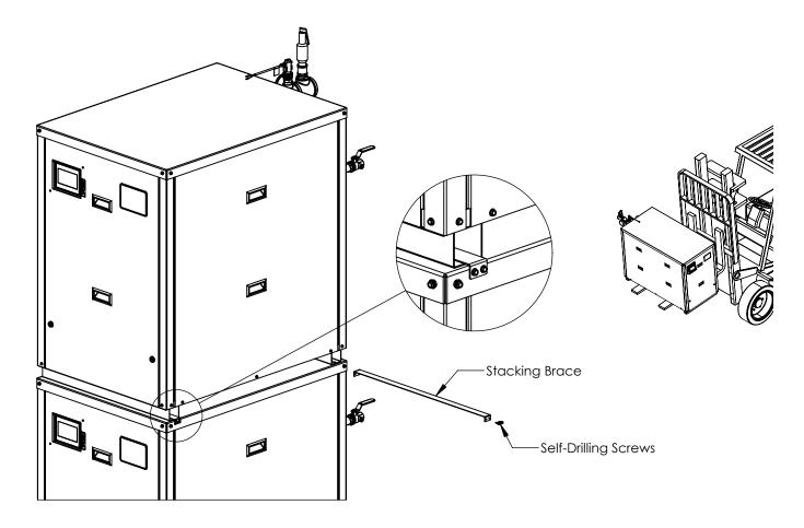
Figure 8: Lifting and Stacked Mounting
