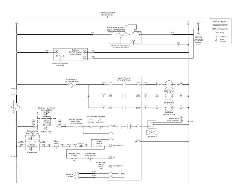
Figure 31: 1250-1500 Wire Diagram
