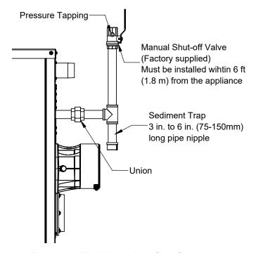
Figure 23: Field Installed Gas Connection
