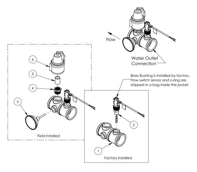
Figure 18: Relief Valve Package Assembly
