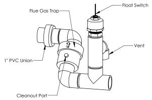
Figure 17: Condensate Drain Assembly
