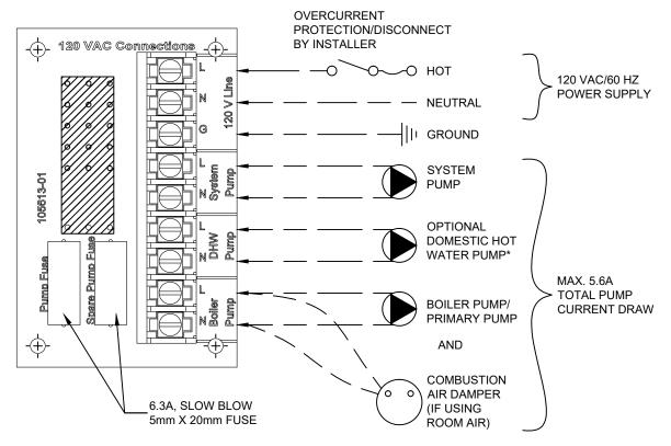
\* For indirect water heating with boiler models. Use Primary Pump for direct water heating with water heater models.
