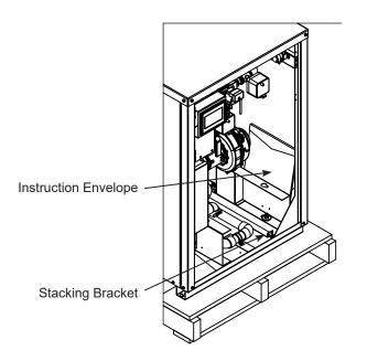
Figure 4: Loosely shipped parts locations
