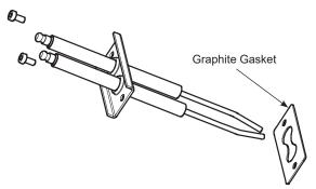
Figure 34: Ignition Electrode Assembly
