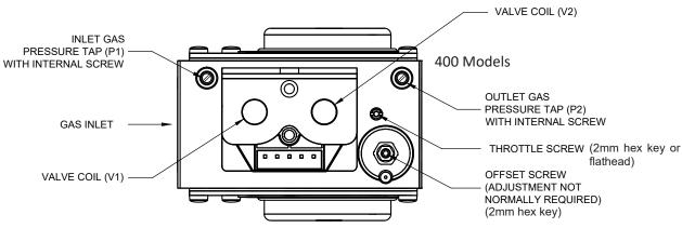
Figure 33: Gas Valve Adjustment
