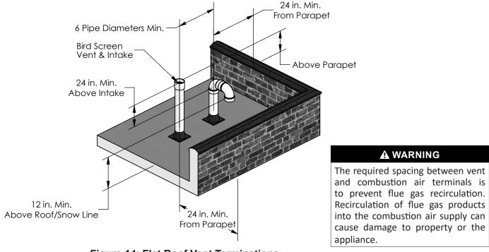
**Figure 14: Flat Roof Vent Terminations**
