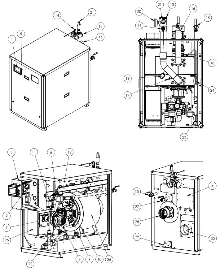
Figure 5: Component Identification
