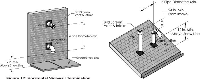
**Figure 12: Horizontal Sidewall Termination**
