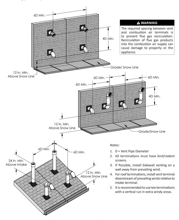
Figure 15: Multiple Appliance Direct Vent Termination
